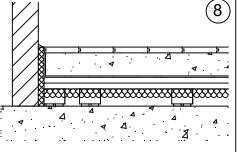
Trim excess Perimeter Isolation Strip at or below the level of the finish flooring. Caulk using an acoustical sealant.
