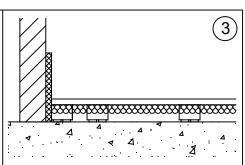
Place the first row of SoundPanel starting in one corner of the room. Start the next row of SoundPanel offset by 16". Cut the first SoundPanel of every other row, then continue with full panels.
