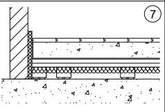
After the concrete has cured, remove excess poly sheeting and install finish flooring as recommended by the flooring manufacturer.
