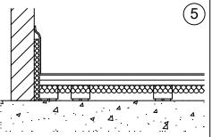
Cover the floor and Perimeter Isolation Strips completely with 2 layers of 6-mil poly sheeting. Seams of sheeting should overlap by at least 4". Tape all seams to prevent concrete from leaking through.
