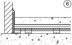
Place reinforcement and pour floating slab in place as per project design and specification.
