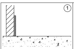
Tape Regupol Perimeter Isolation Strip in place, continuously on all adjoining strucutral elements, such as walls, columns, and protrusions.
