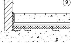
Leave a slight gap between the baseboard and the finished floor. Avoid any rigid connections between the isolated floating floor and adjacent structural elements.
