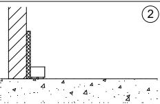
Place Regupol SoundPad butt-joined to the perimeter of the room, around all structural elements. Individual SoundPad should be spaced equal to or less than 16".
