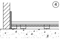
Install 2nd layer of 1/2" OSB or plywood over top of SoundPanel, staggered, so that the seams do not line up. Glue and fasten with trowel, wood glue, 1" screws, 6" o.c. along perimeter, and 8" o.c. throughout.
